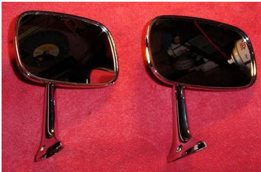
6. After the JBWeld and Epoxy have completely cured, apply a RTV primer (Locktite or Permatex brand) to both glass and the 4 housing posts where contact will be made. Then apply a good bead of RTV to each of the 4 posts and press the mirror glass into place. Put a thick, clean rag
